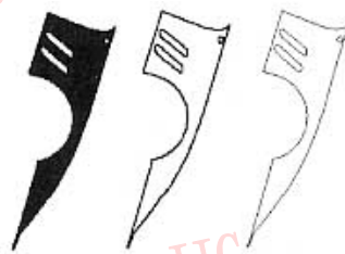
图 11 同时具有内边界和外边界的点云数据边界提取 Fig. 11 Boundary extraction of point cloud with inner and outer loop boundary
